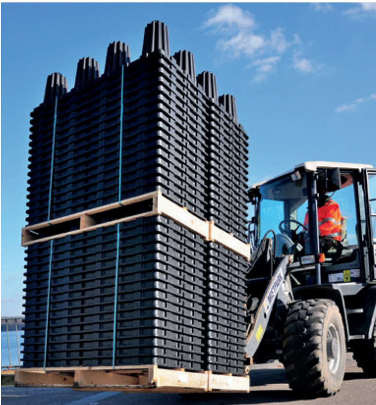
The modular ACO Stormbrixx infiltration system reduces transport costs and therefore more than halves CO 2 consumption and the storage space required in storerooms and on the construction site compared to other systems
